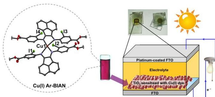
**Figure 1** Incorporation of panchromatic Cu(I) chromophores in dye-sensitized solar cells.
