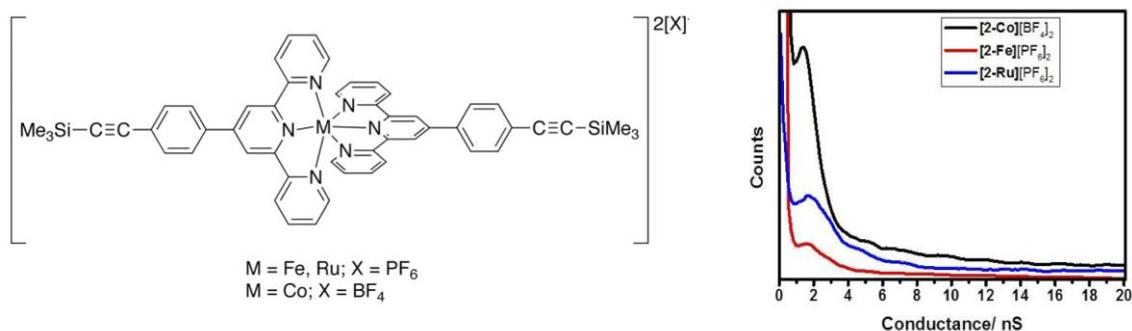
**Figure 1** An example of a family of 'wire-like' coordination complexes and conductance histograms.
